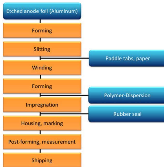
Fig. 6: Manufacturing process of polymer aluminum electrolytic capacitors
