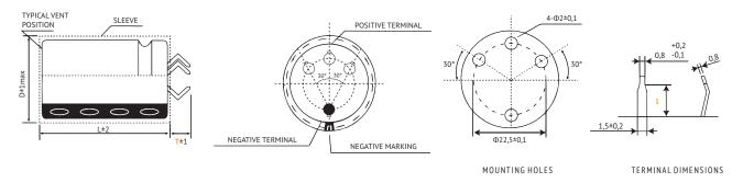
For  $\emptyset D \geqslant 30$ mm only. Other terminal types and styles on request. For diameter  $\emptyset D \geqslant 45$ mm the safety vent is typically placed at the side of the housing.
