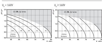
$I_{_{\rm A}}$  = actual ripple current at 120Hz,  $I_{_{\rm R}}^{}$  = rated ripple current at 120Hz, 85°C Multiplier of Useful Life as a function of ambient temperature & ripple current load
