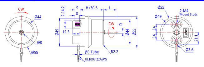
Indication of Letters: D: Shaft Diameter L: Shaft Extended Length H: Stator Lamination Height **Remarks**: 1) Only the dimensions marked in letters are changeable as needed. Other dimensions are fixed.
