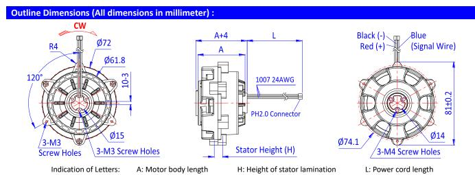
Remarks: 1) Only the dimensions marked in letters are changeable as needed. Other dimensions are fixed.2) The height and the shape of the above motor body are not changeable unless we open new moulds.
