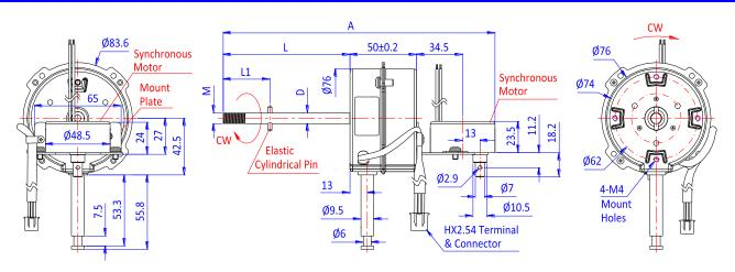
Indication of Letters: D: Shaft Diameter L: Shaft Extended Length A: Motor Body Total Length Remarks: 1) Only the dimensions marked in letters are changeable as needed. Other dimensions are fixed.
