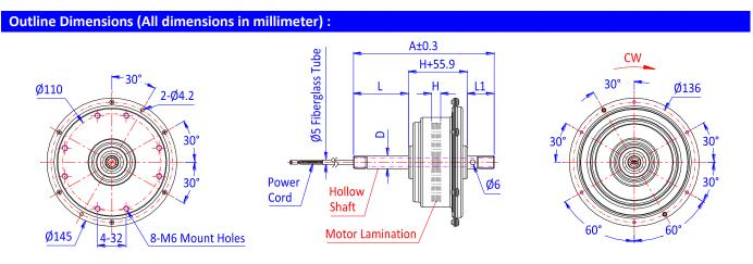
A: Shaft Total Length D: Shaft Diameter H: Lamination Height L: Rear Side Shaft Extended Length L1: Front Side Shaft Extended Length Remarks: 1) Only the dimensions marked in letters are changeable as needed. Other dimensions are fixed.
